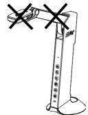
■ Do not pull the camera arm and camera part in the opposite direction.
